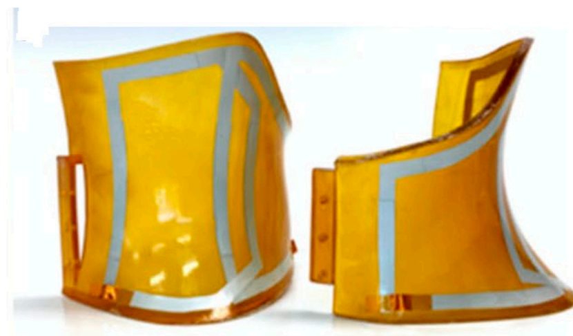
Figure 11. A custom coil array designed for covering the entire neck surface area. Reprinted from [67], 2021, Springer.
