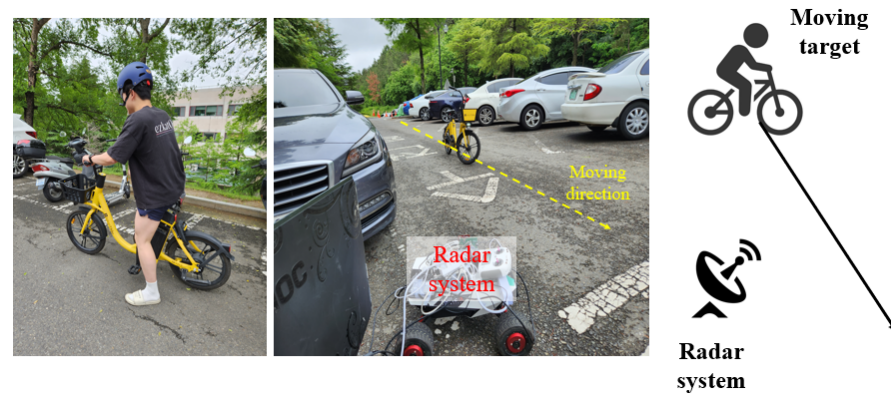
Figure 19. Outdoor FMCW radar experimental environment and configuration (case 3).
