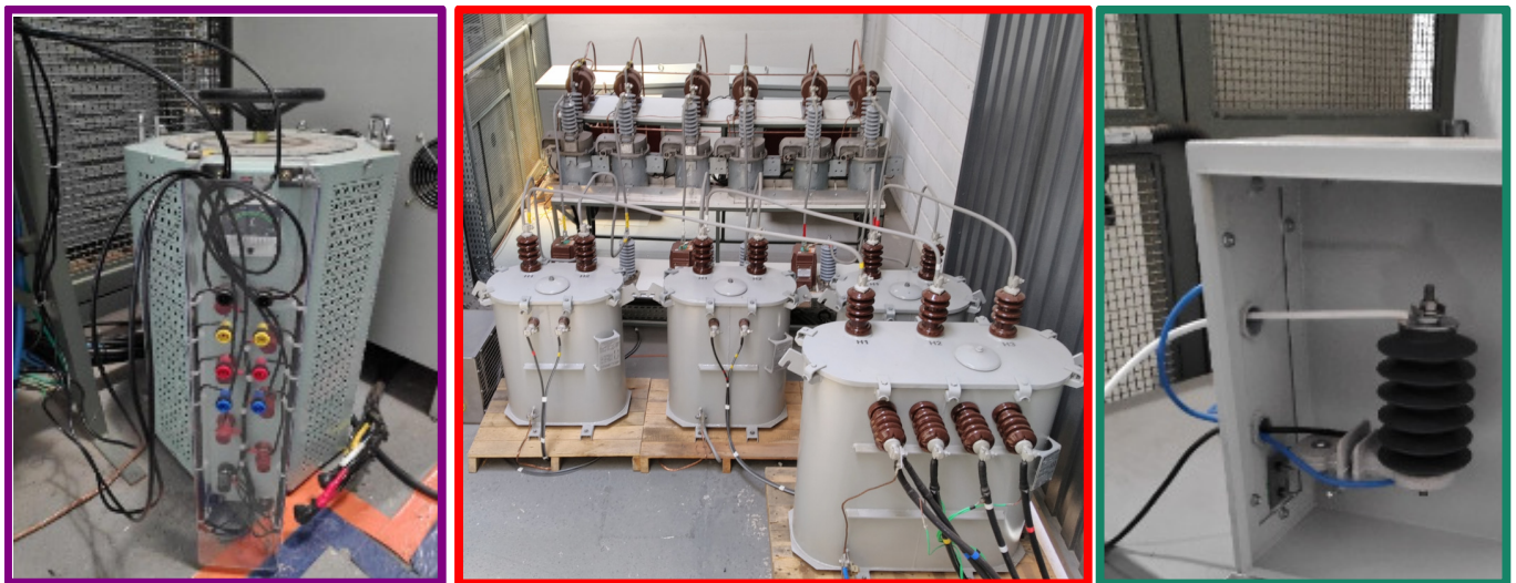
Figure 5. Photograph of the accelerated aging test setup (low voltage VARIAC—medium voltage test substation—arrester that was aged).
