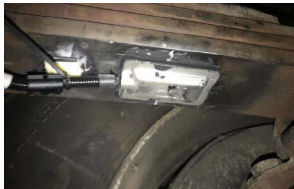
Figure 12. Wheel dynamic vertical load sensor installation diagram.
