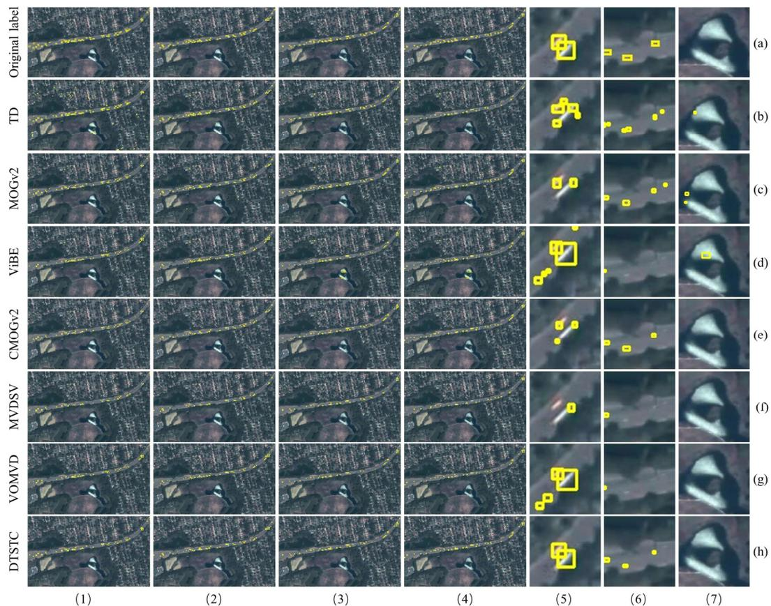
**Figure 9.** Comparison diagram for Area 1 moving vehicle detection, where columns (1)–(4) are the detection results in Area 1 for frames 30, 50, 70, and 82, respectively. Columns (5) and (6) show the road area refinement maps. Column (7) shows the refinement of the background area. The yellow box in the diagram shows the detected moving vehicles. For ease of description in the subsequent text, the names of the methods are replaced by (a–h).
