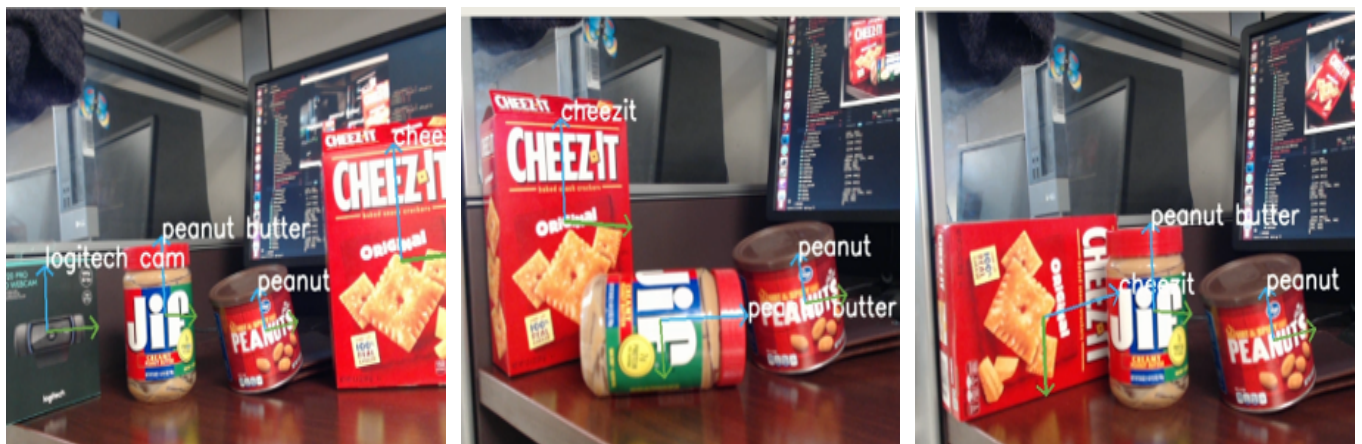
Figure 15. Multiple object detection with estimated planar vectors.
