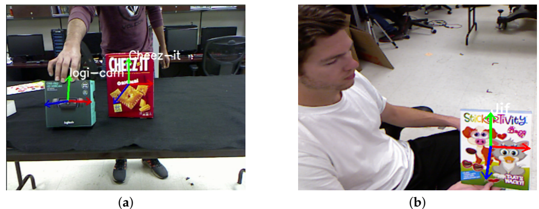
Figure 17. Pose estimation performance: (a) Pose estimation of multiple objects; and (b) Estimated pose of an object held by a human.
