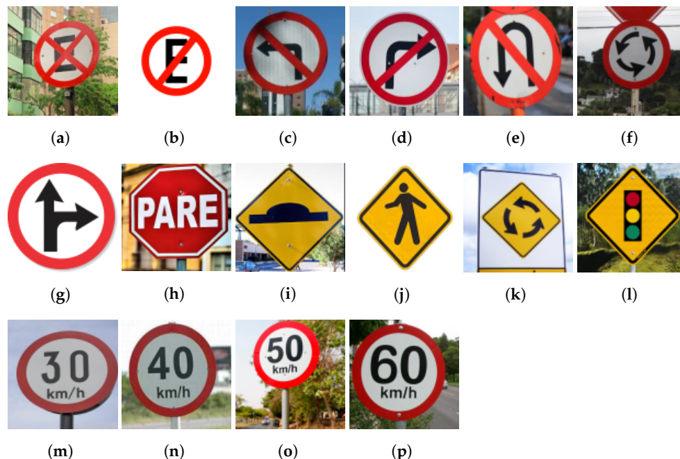
Figure 1. (a) No Stopping or Parking. (b) No Parking. (c) No Turning Left. (d) No Turning Right. (e) No U-turn Left (f) Roundabout Ahead. (g) Right Turn or Straight Only. (h) Brazilian Stop. (i) Speed Bump Ahead. (j) Pedestrian Crossing ahead. (k) Roundabout Ahead. (l) Traffic Lights Ahead. (m) 30 km/h Speed Limit. (n) 40 km/h Speed Limit. (o) 50 km/h Speed Limit. (p) 60 km/h Speed Limit.
