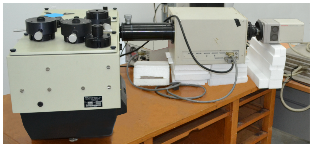
Figure 14. Visible range spectroscopy setup.
