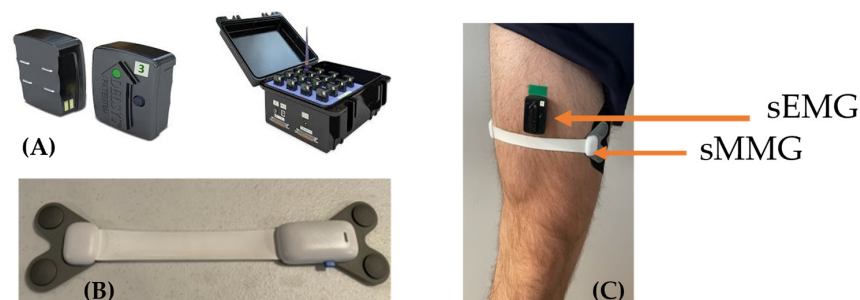
Figure 1. sEMG (A) and sMMG (B) sensor placement across the quadriceps muscle (C).
