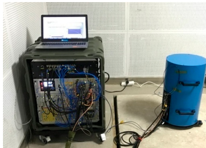
Figure 2. The Photo of the compact ^{85}\text{Rb} atom gravimeter.
