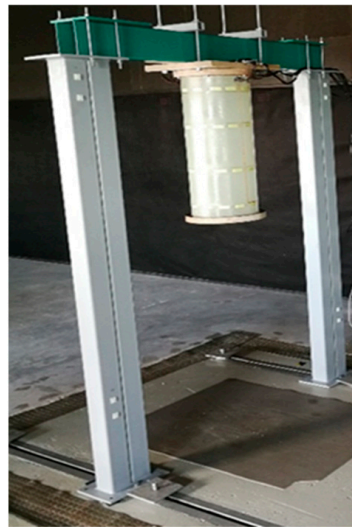
Figure 6. Modal test stand.
