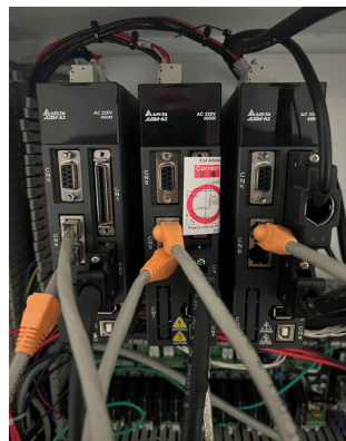
Figure 3. Delta ASDA-A2 servo drive.
