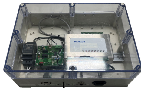
Figure 4. BALTech DAQ-204 vibration module.
