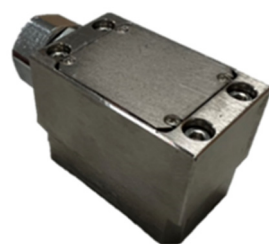
Figure 5. Picture of the BT-1513 triaxial accelerometer.
