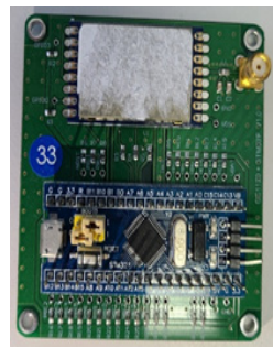
Figure 4. Transceiver configured with STM32F103 + CC1120.
