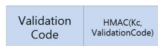
Figure 6. ReturnTicket structure that is configured when a validation code has an error.
