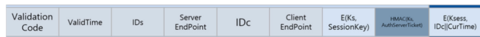
Figure 9. Request or SubscribeEventGroup structure that a client configures to pass AuthServerTicket and FreshnessToken to a server.
