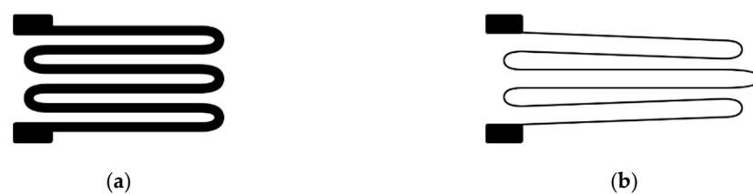
Figure 4. Diagram showing the physical behavior of a strain gauge. When a force is applied, it stretches, increasing its electrical resistance. (a) Strain gauge at rest position, broader tracks and better conductivity; (b) strain gauge in a stressed position, narrower tracks increase electrical resistance and decrease conductivity.
