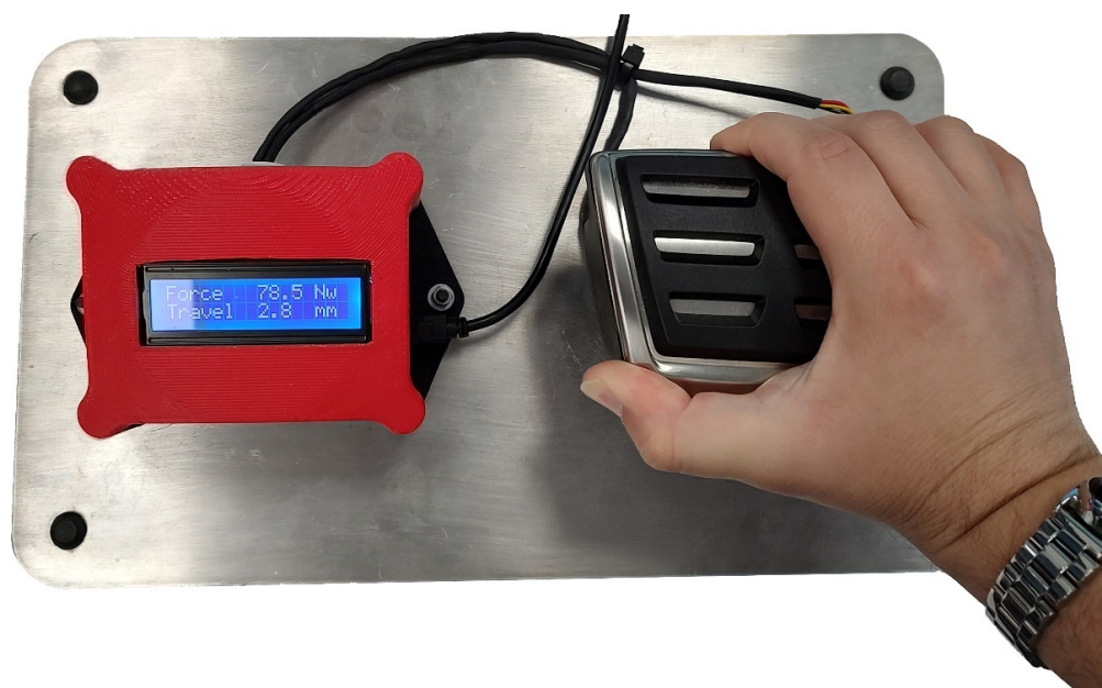
Figure 13. Electronic braking pad prototype. Force is applied to the pedal, and sensor readings are updated on the LCD.
