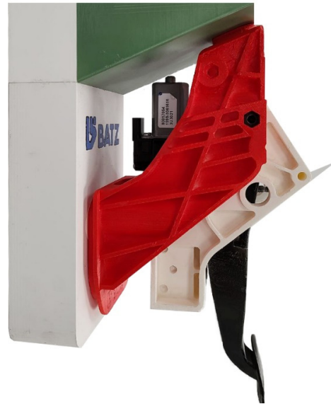
Figure 10. Retractable prototype. An actuator allows the pedal to retract to a flat position in 5 s.
