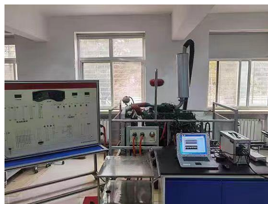
Figure 8. Diesel engine condition monitoring test bench.
