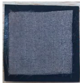
Figure 4. The sensor prepared using hot press welding.
