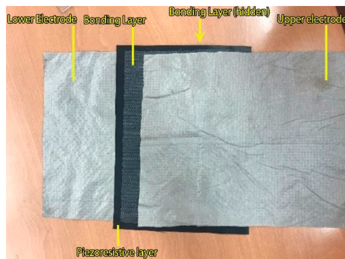
Figure 6. The large-scale sensor prepared using bonding material.
