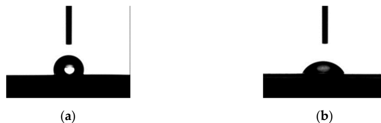
Figure 15. Contact angle (a) before plasma treatment, (b) after plasma treatment.
