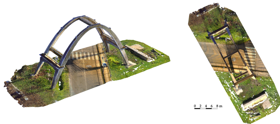
Figure 3. Two views of the LiDAR point cloud derived from the registration of the 19 acquired scans.
