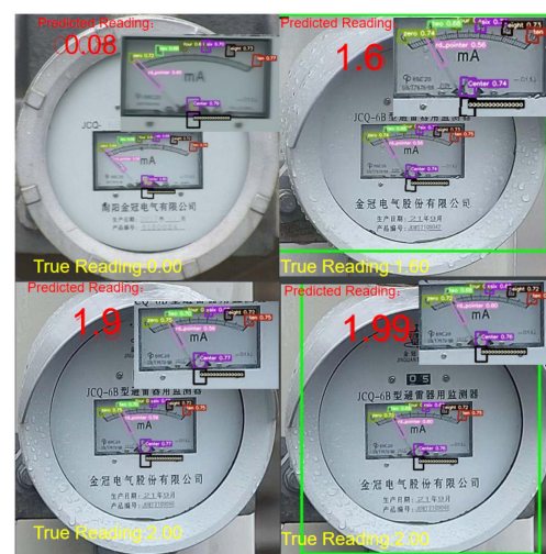
Figure 6. The recognition effect of the YOLOv5-MR model. Predicted-Reading represents the predicted reading, and True Reading represents the actual reading. In the rectangular box in the center of the index dial, the green number 2 represents the scale value 2, the yellow number 0 and 4 represents the scale value 0 and 4, the purple number 6 represents the scale value 6, the black number 8 represents the scale value 8, and the red number 10 represents the scale value 10. The purple center represents the predicted dial center, and the black 000...0 represents the true center of the dial.
