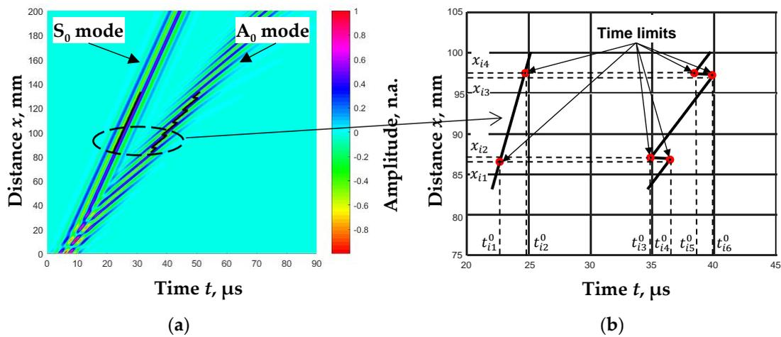
**Figure 2.** B-scan image of the simulated Lamb wave mode signals (color-coded) and calculated zero-crossing instances (line) (a) and zero-crossing instances of the  $i$ -th filter in the narrow range (b).
