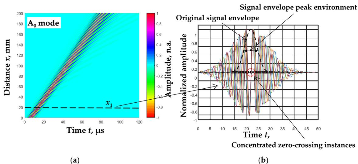
**Figure 1.** B-scan image of the simulated Lamb wave  $A_0$  mode in  $d = 1$  mm thickness aluminum plate at  $f_{ex} = 300$  kHz excitation frequency [24] (a) and signal filtered by five filters (color curves) at the distances  $x_1 = 20$  mm (b).
