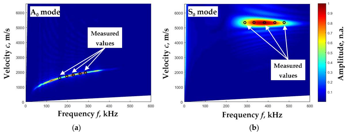
**Figure 10.** Phase velocity dispersion curves of  $A_0$  (a) and  $S_0$  (b) modes were calculated using the 2D-FFT method (color), and phase velocity values were calculated from experimental data using the proposed algorithm (dots).
