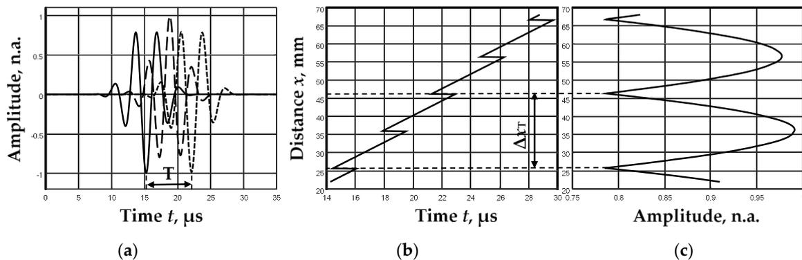
Figure 6.  $A_0$  mode signals at different distances (a), zero-crossing instances in the selected range of distances (b), and the amplitude distribution of the envelope maxima of these signals (c).
