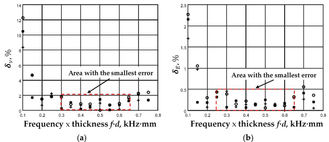
**Figure 8.** Relative error calculations result using different excitation frequencies  $f_{ex}$  and ratios of the amplitudes of  $A_0$  and  $S_0$  modes: 'o'— $L_S = 1$ , '+'— $L_S = 0.5$ ; '\*'— $L_S = 0.1$ . (a) Relative errors of Poisson's ratio calculations; (b) relative errors of Young's modulus calculations.
