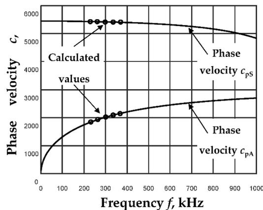
**Figure 3.** Dispersion curves were calculated using the analytical method (lines), and values of phase velocities were calculated for the proposed algorithm (dots) for  $d = 2$  mm thickness aluminum plate at  $f_{\text{ex}} = 300$  kHz excitation frequency.
