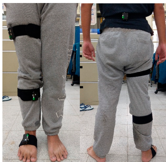
Figure 1. The front and back views of the subject wearing STT-IWS sensors on the sacrum, right thigh, right calf, and right foot of the right leg.
