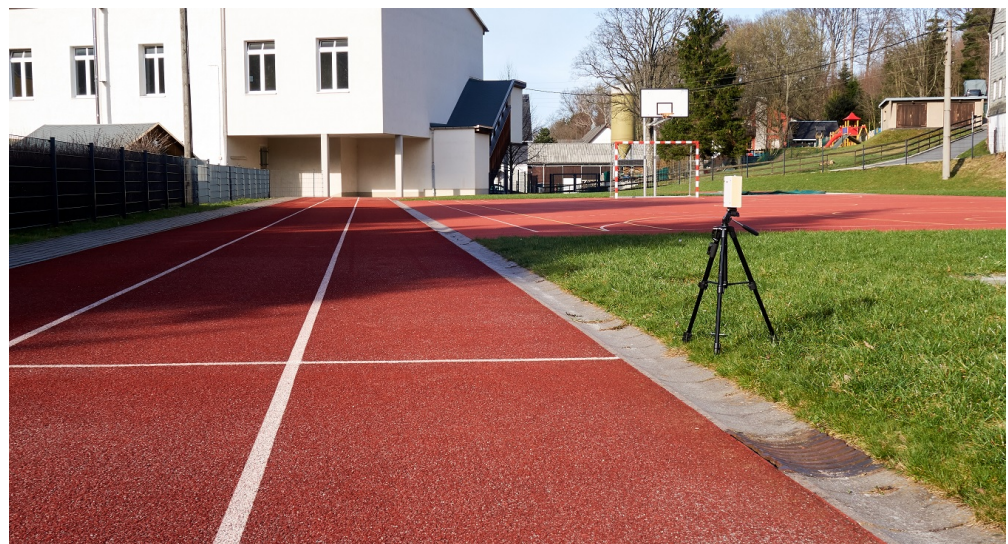
Figure 3. Our camera-based photoelectric barrier can be easily placed on a tripod. Unlike traditional systems, no reflector is required, which greatly reduces setup time. Bluetooth communication eliminates the need for wires.
