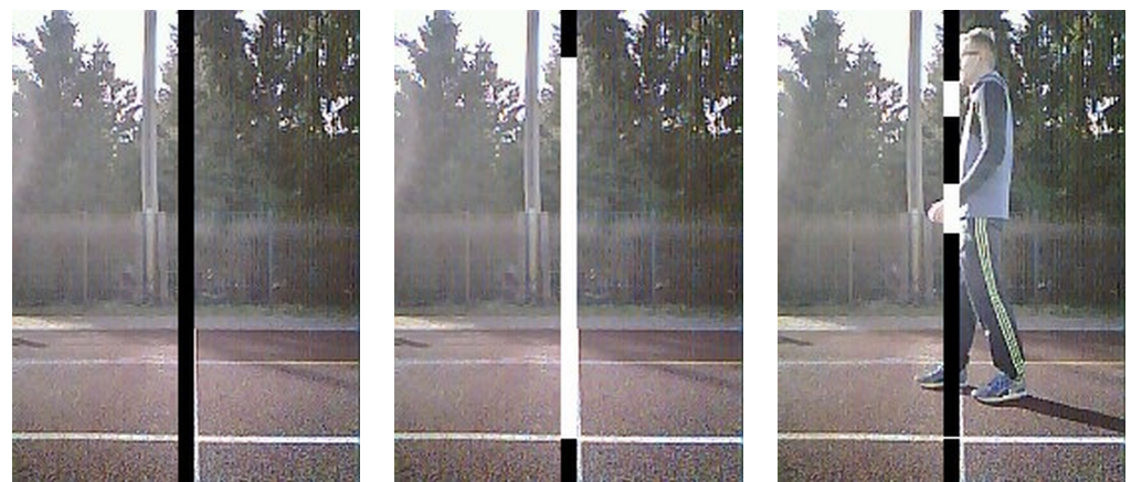
Figure 1. Camera footage with the detection area shown in black and the white areas marking regions, where the image-to-image error is actually calculated. Left: Full virtual barrier. Middle: Default virtual barrier in white. Right: Multi-barrier setting.
