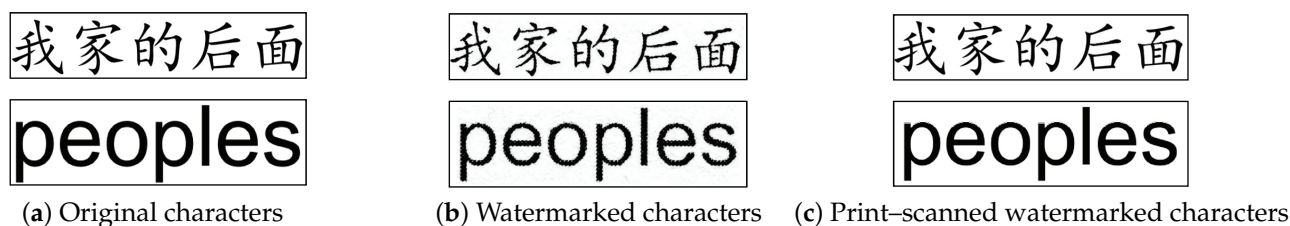
Figure 1. Comparison of original characters, watermarked characters and print–scanned watermarked characters. (a) (top): Chinese characters meaning “the back of my house”, (bottom): English characters; (b) watermarked characters corresponding to (a); (c) printed-scanned watermarked characters corresponding to (a).
