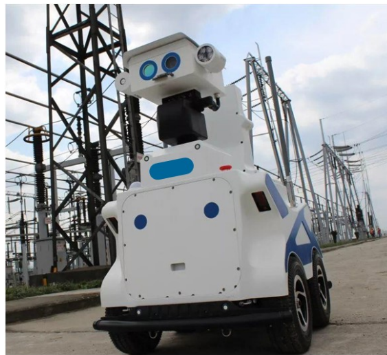
Figure 2. Substation inspection robot from a Chinese company.
