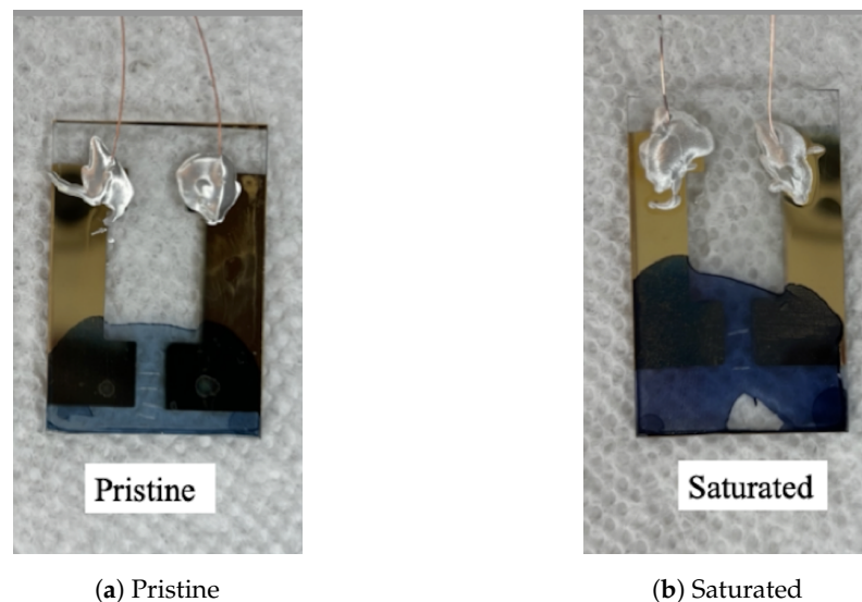
Figure 6. (a) Pristine PEDOT:Tos film (light blue) versus (b) fully saturated PEDOT:Tos film (dark blue).
