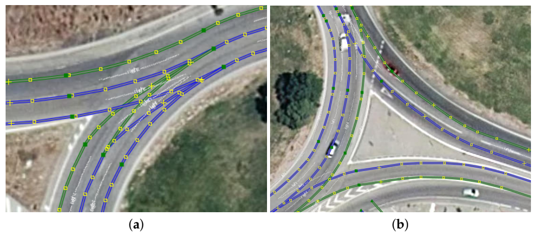
Figure 5. Lanelets from OSM drawbacks. (a) Misalignment. (b) Wrong number of lanes.
