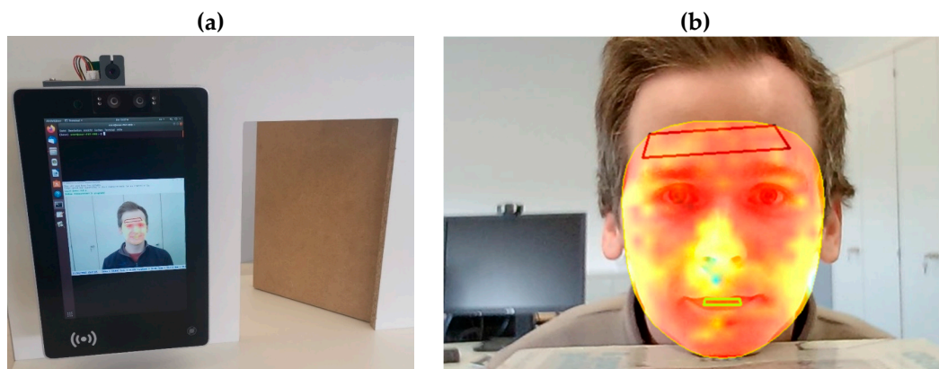
Figure 7. (a): System prototype; (b): exemplary illustration of the combined sensor data fusion with facial region detection and tracking.
