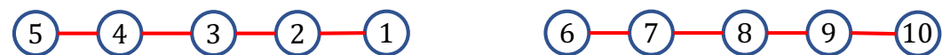
Figure 6. Graph connection topology of Formation-1. Mobile agents are connected only with their neighboring agents. The red line shows the connection between the agents.
