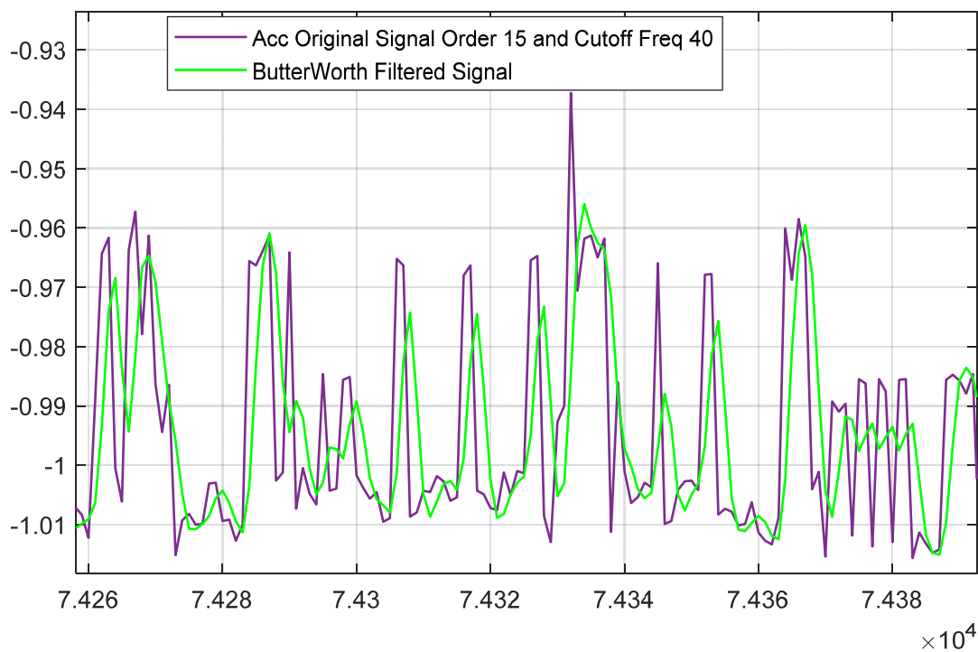
Figure 2. Sample signals after filters applied for motion sensor data.
