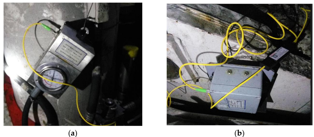
Figure 3. Hydraulic support status sensing sensor. (a) FBG inclination sensor; (b) FBG pressure sensor.
