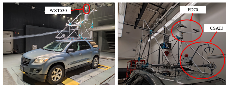
Figure 2. The WoW vehicle used for field measurements.
