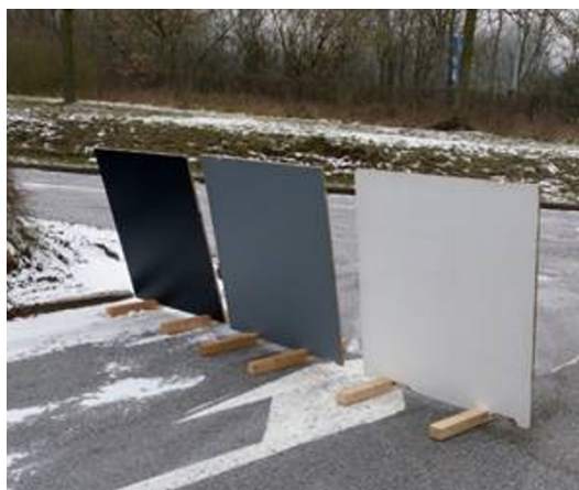
Figure 7. This figure shows the controlled environment for a second denoising experiment. The setup consists of 3 boards of different colours with known reflective properties and positioned at a distance of 100 m from the real-world LiDAR. Point clouds are captured and denoised using a neural network trained on synthetic data generated by our digital twin. Denoising results are shown in Table 2.
