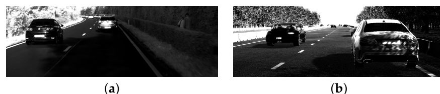
Figure 11. Comparison between images captured by the CMOS sensor of our real-world LiDAR (a) and its digital twin (b). Though the synthetic images are not used during training, they clearly demonstrate the resemblance of the output of the proposed digital twin and the real-world device. Resolution, field-of-view, sensor sensitivity, LiDAR position, and orientation are all accounted for during simulation, which is mandatory for successfully training neural networks operating on real data.
