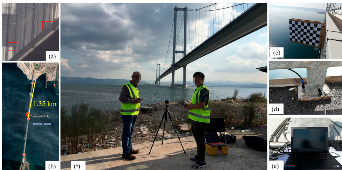
Figure 15. Experimental setup of the first experiment of the Osman Gazi Bridge: (a) image from camera (The red boxes, from left to right, indicate the static point and the installed chessboard, respectively), (b) camera location in map, (c) wooden chessboard, (d) accelerometers in vertical and horizontal direction, (e) computer for data acquisition, (f) camera setup.
