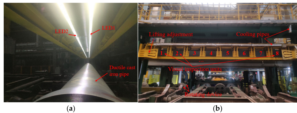
Figure 5. The experimental prototype system at the production site. (a) Local scene; (b) global scene.
