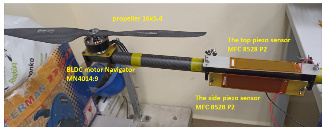
Figure 10. BLDC based drive unit with piezo-sensor.
