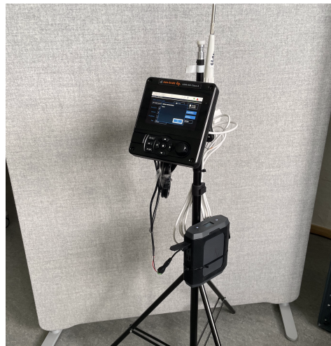
Figure 5. The A200 connected to a battery and a VHF antenna.
