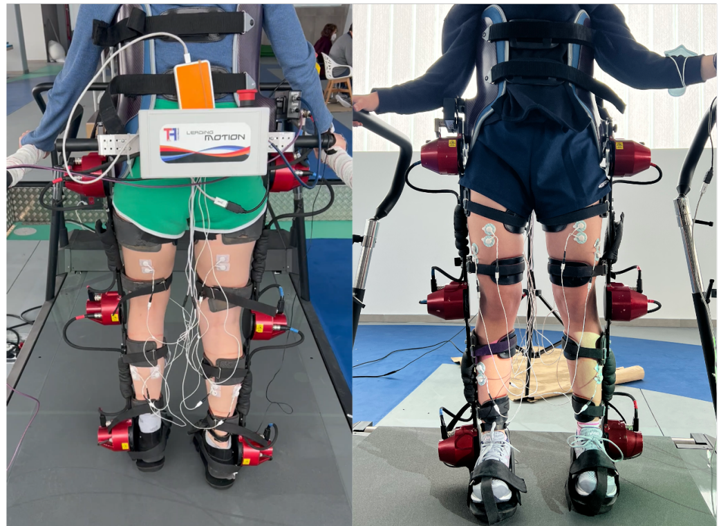
Figure 5. Pictures of two different subjects while they walked with Exo-H3. Most of the experimental setup is represented in the two pictures.
