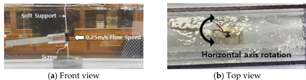
Figure 6. Power efficiency verification model according to axial rotation variable.
