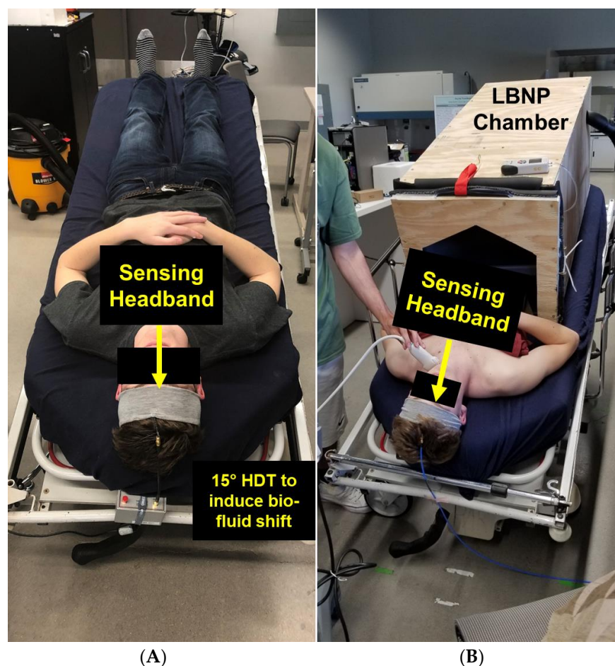
Figure 2. EM skin patch sensor embedded in wearable headband to detect induced bio-fluid shift in (A) 15° head down tilt and (B) during administration of lower body negative pressure (LBNP).
