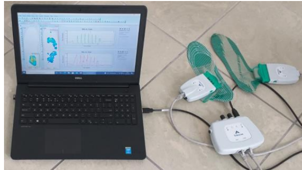
Figure 6. View of the components of the Tekscan F-Scan In-Shoe measurement module.
