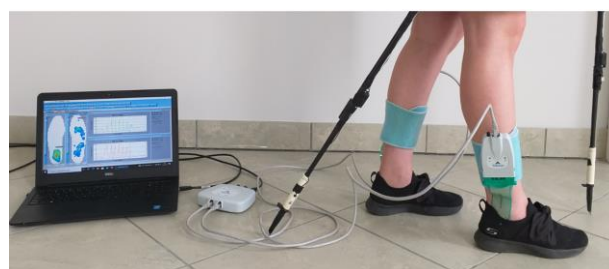
Figure 9. View of a person prepared for a measurement walk with NW poles equipped with elements of the PoleM and F-Scan measurement systems.
