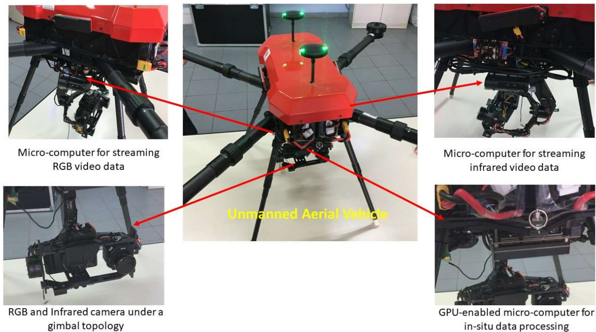
Figure 3. Proposed UAV-based power line inspection platform and key components.
