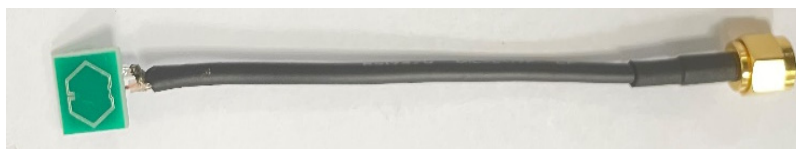
Figure 8. Antenna prototype fed by a 50- \Omega RF mini coaxial cable.
