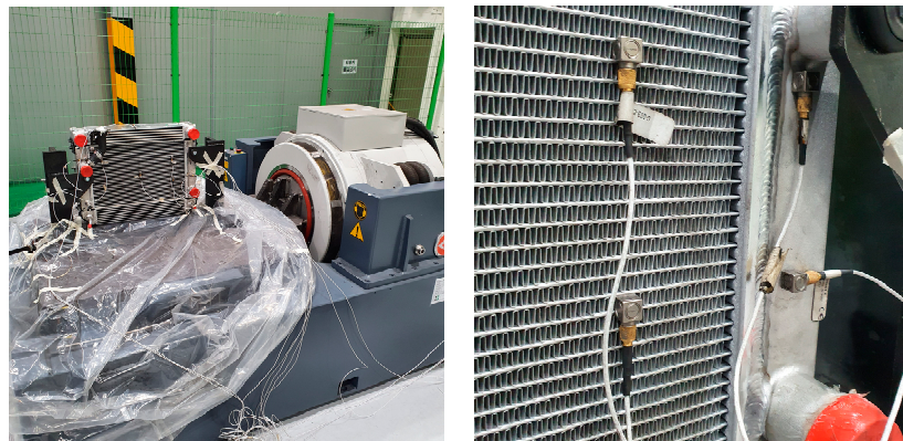
Figure 4. Experimental setup: radiator equipped with acceleration sensors mounted on a vibration dynamo.
