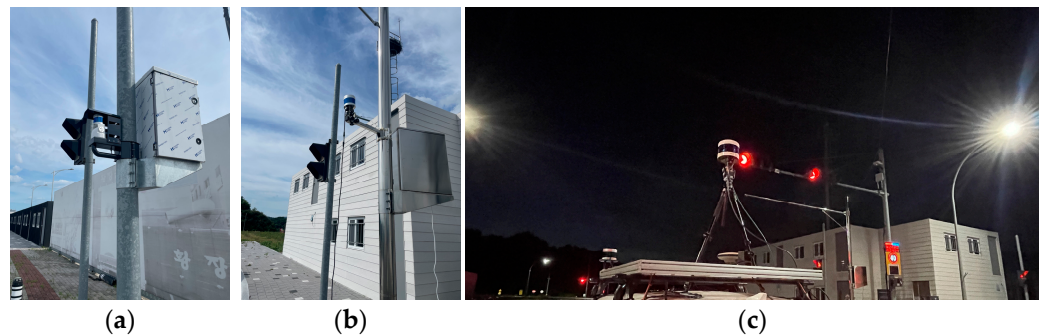
Figure 14. Lidars placed on real environment. (a) First 40-channel lidar. (b) Second 40-channel lidar. (c) The 128-channel lidar.
