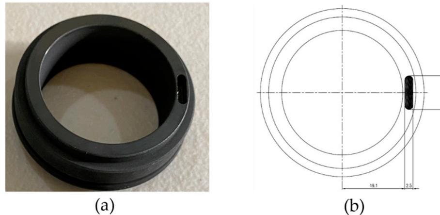
**Figure 10.** (a) Mechanical seal scratch. (b) Schematic diagram of the mechanical seal scratch.
