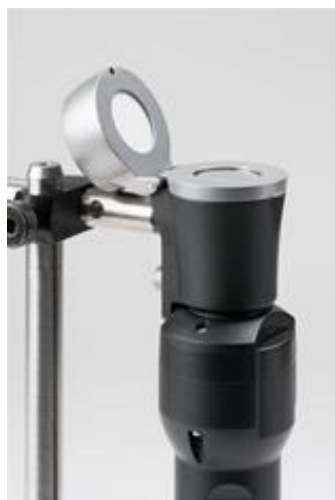
Figure 1. Droplet collar accessory attached to the MicroNIR portable instrument used to analyze the unadulterated and adulterated commercial whisky samples with methanol.
