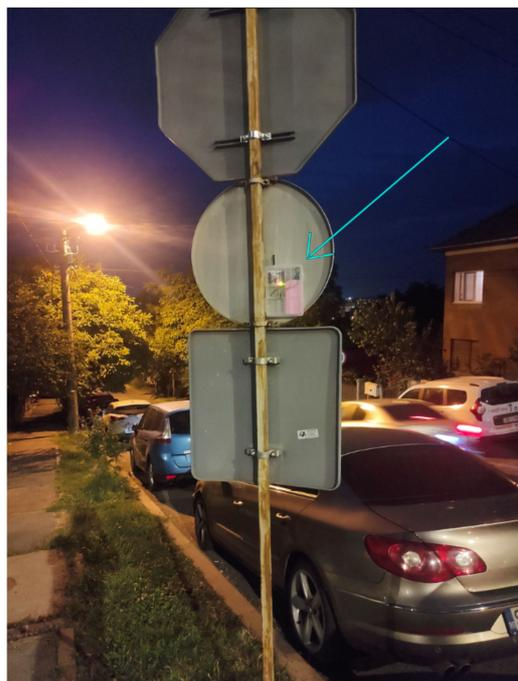
**Figure 9.** End node cluster mounted on signal pole (Highlighted by arrow).
