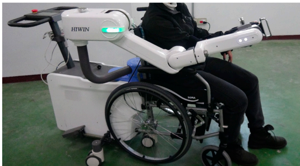
Figure 1. Upper limb rehabilitation robot U100 (permitted via HIWIN Technologies Corp., Taichung City, Taiwan).
