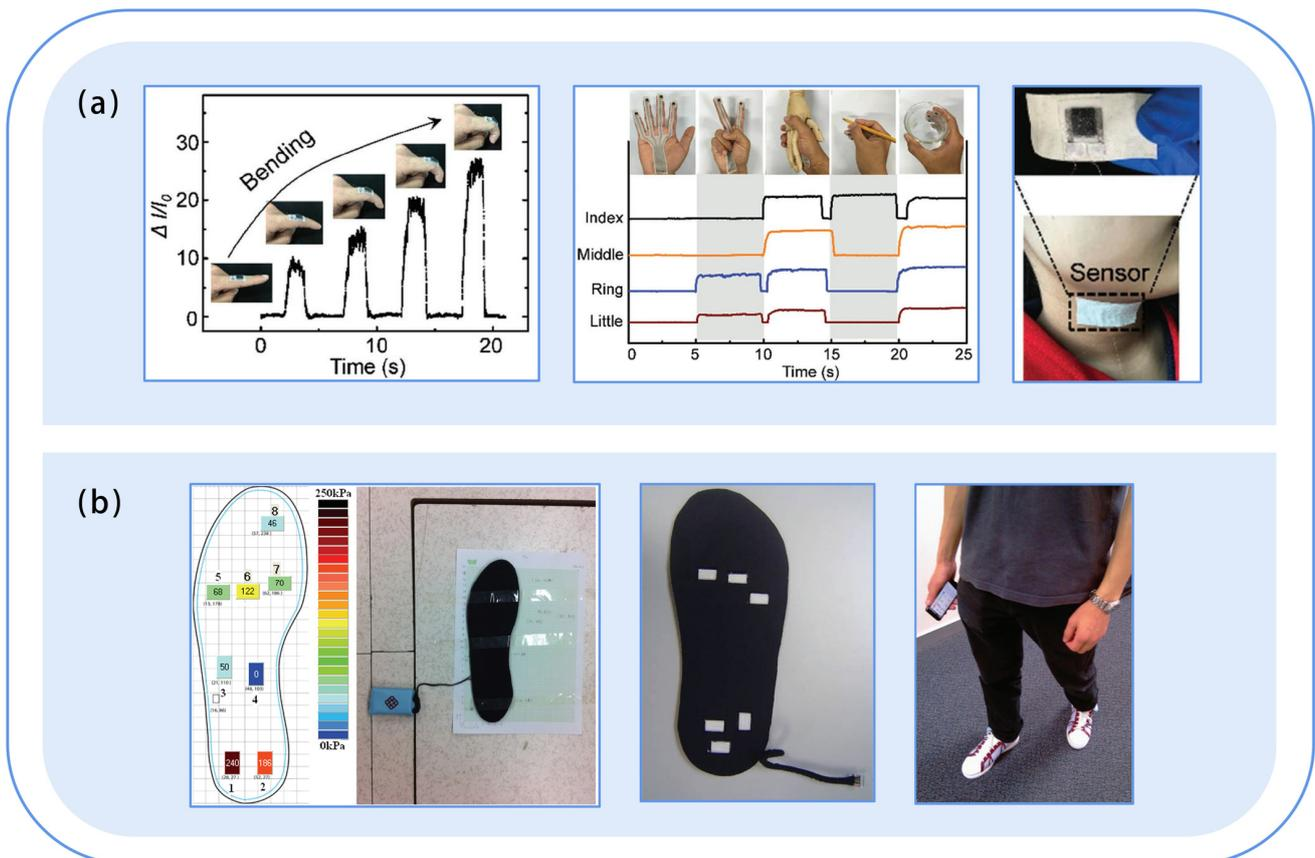
**Figure 9.** Study of flexible pressure sensors in human motion monitoring. (a) Textile sensors attached to the skin of a curved finger to monitor different mechanical forces in real-time. Reproduced with permission [3]. Copyright 2017, John Wiley & Sons; (b) Textile pressure sensor integrated with a shoe insole to monitor plantar pressure distribution and gait analysis [113].
