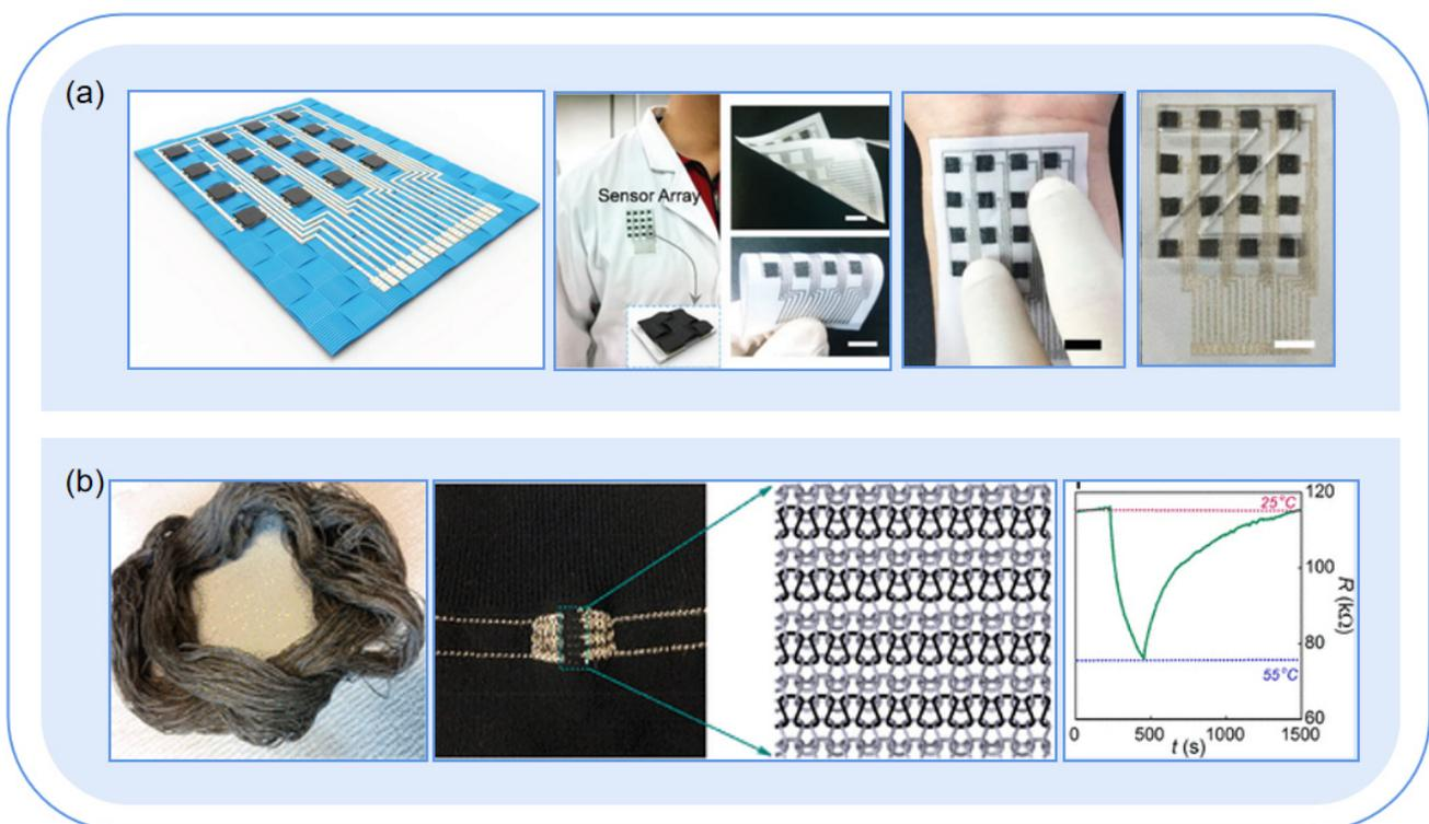
**Figure 7.** Combinations of flexible sensors and fabrics. (a) Coated on the fabric surface. Reproduced with permission [3]. Copyright 2017, John Wiley & Sons; (b) coated on fiber or yarn first, and then knitted into fabric. **Left:** Hank of rGO-dyed (coated) cotton yarn; **Middle:** Knitted temperature sensor with graphene-coated yarn; **Right:** Time response property of the knitted temperature sensor. Reproduced with permission [79]. Copyright 2019, American Chemical Society.
