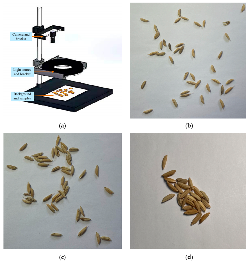
Figure 1. Image acquisition platform and sample images. (a) Mobile phone camera working diagram; (b) sample image of mildly adhered rice grains; (c) sample image of moderately adhered rice grains; (d) sample image of severely adhered rice grains.
